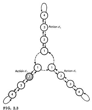
A sequence of such signals sends the device towards the outer edge of a petal to reach the final state where it stays. If a fine signal comes to the input, the state is changed in the direction indicated by the dashed arrows. The device with a sequence of penalties moves inwards until another fine signal causes it to pass over to another petal of the daisy; thus a change of action occurs. As can be shown in Fig. 2.3, these changes occur in a sequential fashion.
